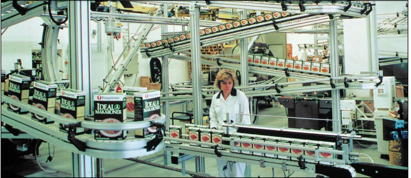
Large FlexLink installation at Kungsörnen macaroni factory
